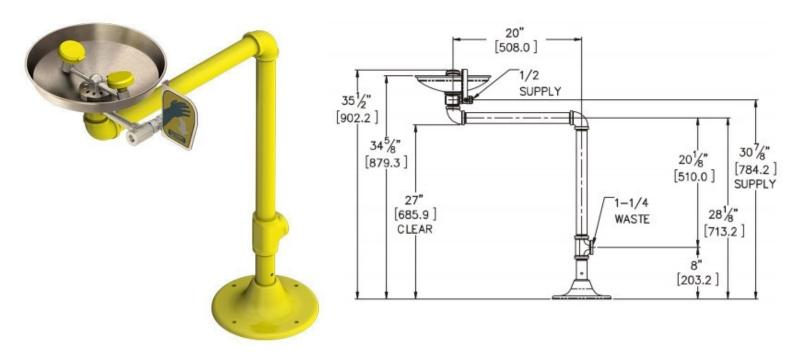
Model S0340-BF is our free standing DDA compliant eye wash with stainless steel bowl. Comes complete with stainless steel bowl, plastic eye/face wash spray heads, an inline strainer and a stay-open 1/2" ball valve with a push handle. Pedestal mounted to allow freedom of being positioned away from walls and DDA compliant so suitable for disabled users.
